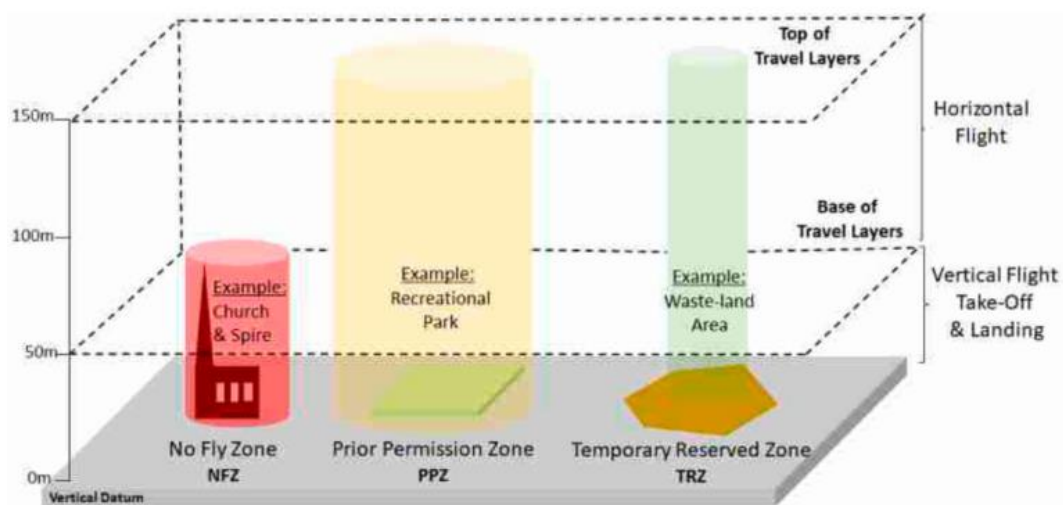
Figure 10: Schematic detailing of No-Fly Zone, Prior Permission Zone and Temporary Reserved Zone (McCarthy et al. 2020).
