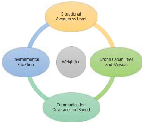
Figure 2. Scheme of the factors which are considered in the Field Theory algorithm
