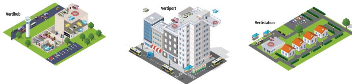
Figure 5: Overview of different types of TOLA infrastructures for VTOL aircraft [21].
